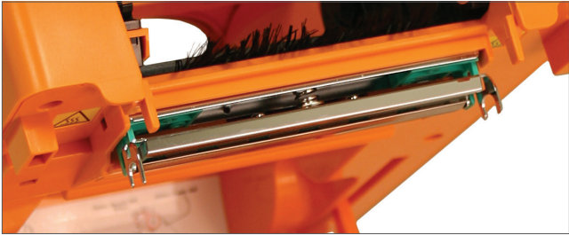
Figure 1 The print head includes the entire metal bar that sits under the printer cover.
