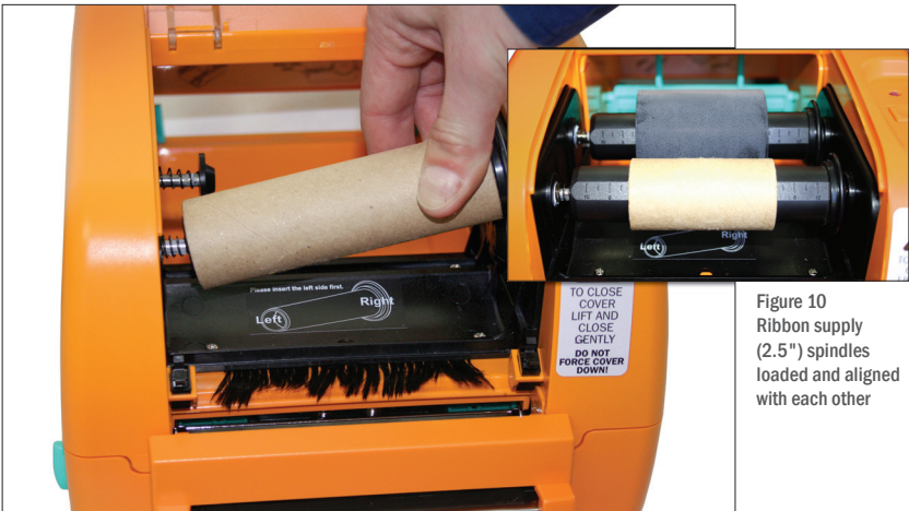
Figure 9 Ribbon rewind spindle with paper core (4.3") being applied to the front spring-loaded hub
