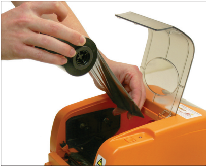
Figure 7 Ribbon supply (4.3") spindle being inserted at rear hubs
