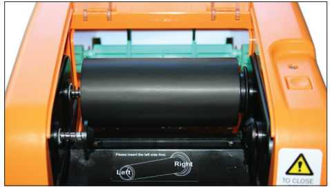
Figure 8 Ribbon supply (4.3") spindle inserted at rear hubs
