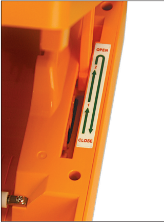
Figure 5 Lift printer cover all the way up, then press down until it latches shut.
