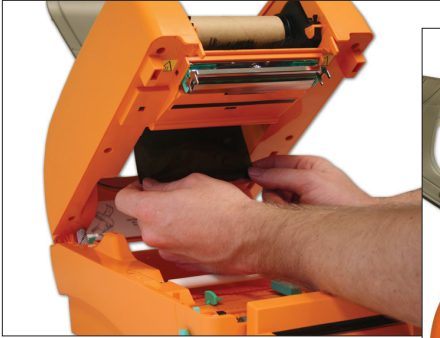
Figure 12 Ribbon supply (4.3") being pulled down
