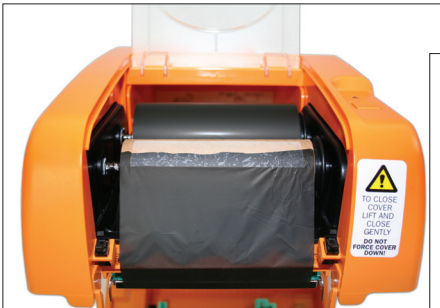
Figure 14 Ribbon supply (4.3") taped to ribbon rewind spindle
