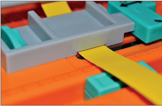
Figure 10 Supply aligned under tape guide and over media sensor
