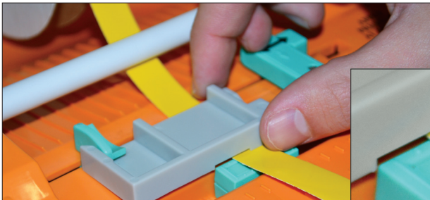
Figure 7 Align supply in the grooved section for easy movement.
