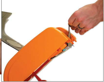
Figure 13 Ribbon supply (4.3") being pulled up to the ribbon rewind spindle
