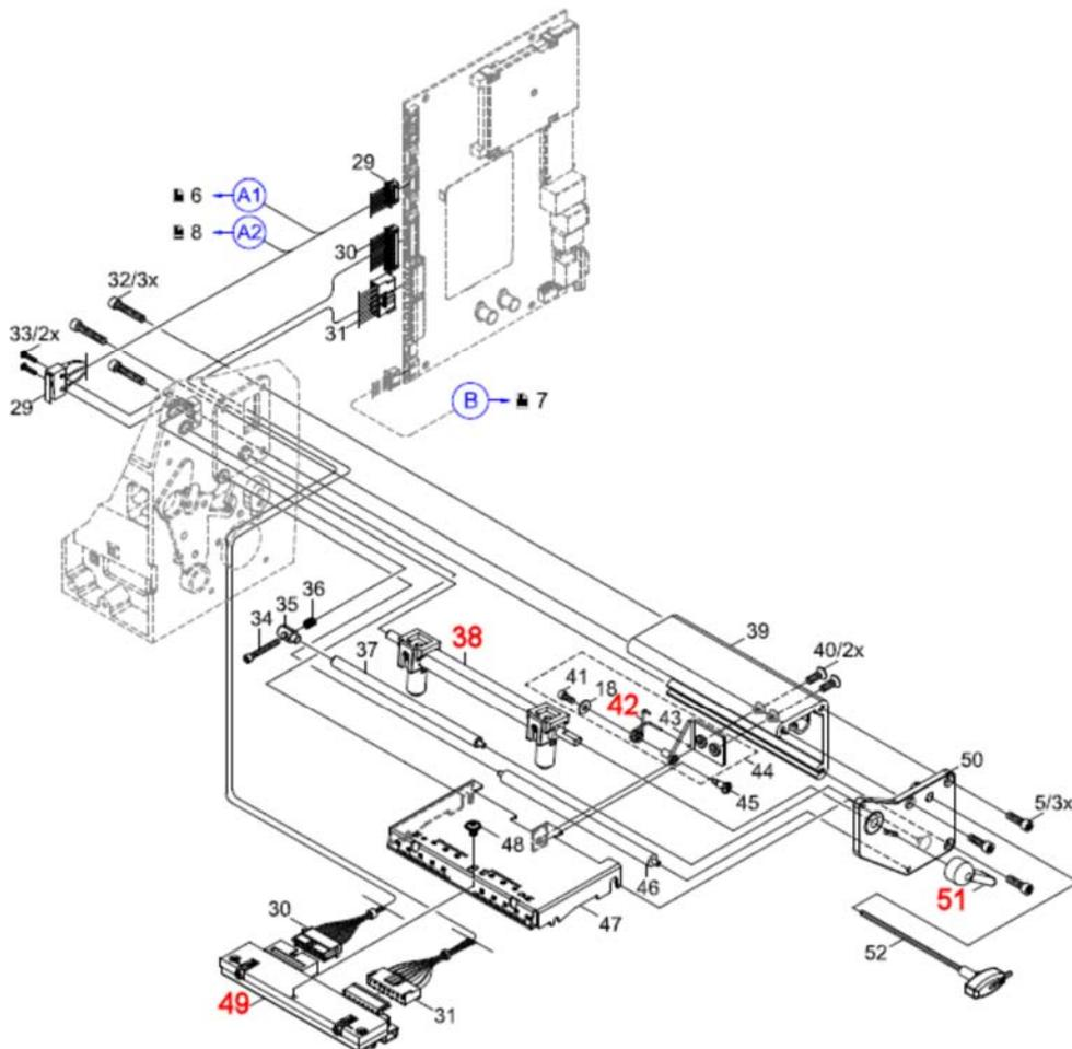
Figure 5 – TE3112/TE3124-PRINTER (print head/mechanical)
