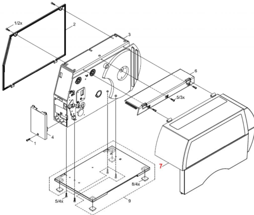
Figure 3 - TE3112/TE3124-PRINTER (cover)
