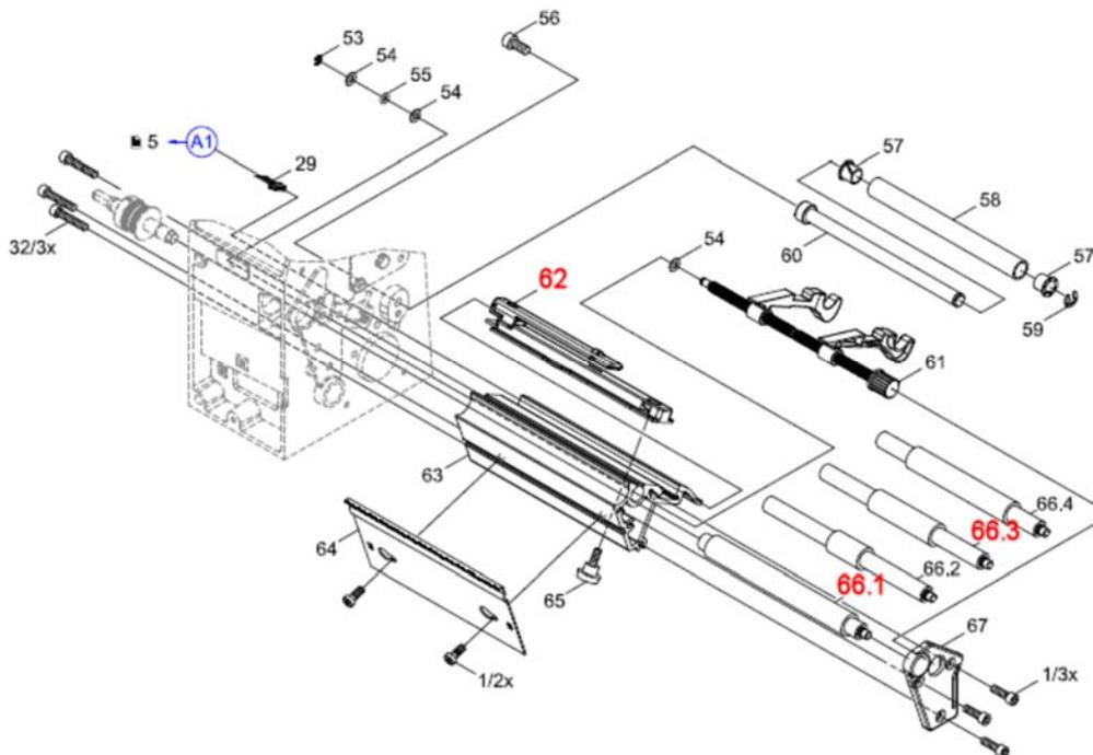
Figure 6 - TE3112/TE3124-PRINTER (drive rollers/Sensor)
