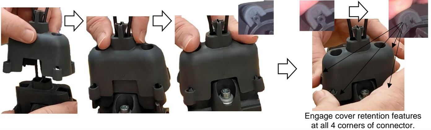
**STEP 5a: Separate TOP HALF and BOTTOM HALF Connector and position over Phase (Run) Wire**
