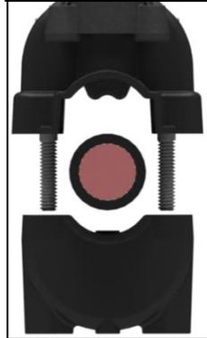
Use 3/16" Allen (hex) drive, tighten fasteners with equal rotation and movement on both sides of wire. Always keep wire centered. Hand-tighten until wire is held firmly and contact starts to press into wire insulation.
