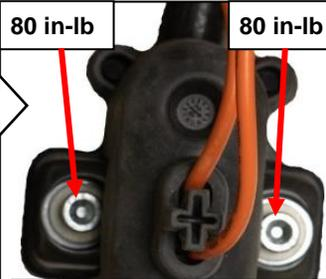
At 80 in-lb, hold torque for 5 seconds on each fastener. Installation is complete. STOP.
