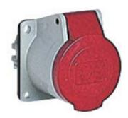
Flush-mounting socket outlet, PLUSO series, 3 poles + N + PE, 6 h (red), 16 A,  $380 \div 415 \text{ V}$ , straight
