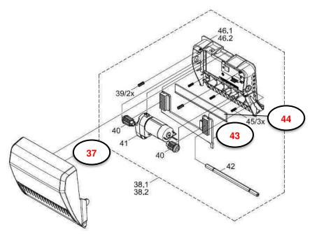
Figure 3 - T2212-PRINTER CUTTER/PERFORATOR
