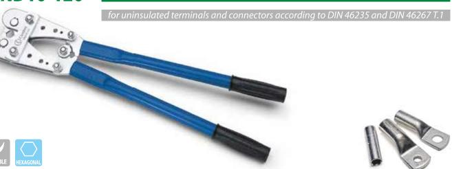
Mechanical tools equipped with rotating dies with hexagonal imprint compliant with DIN 480863 suitable to crimp Copper lugs according to DIN 46235 and through connectors according to DIN 46267 T.1 (refer to page 36-37), particularly sturdy and easy to handle.
