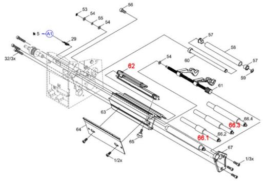
Figure 6 – TE3112/TE3124-PRINTER (drive rollers/Sensor)
