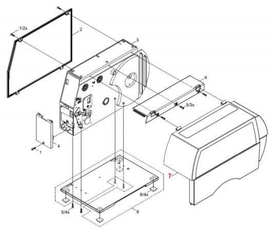
Figure 3 – TE3112/TE3124-PRINTER (cover)
