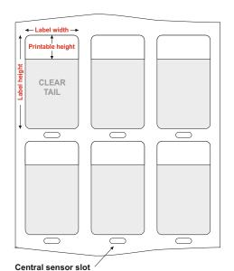
ESL self laminating labels are supplied with a centred senor slot for ease of loading in printer for printing.
