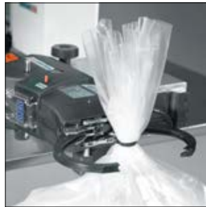
Packaging application with Bench mount kit horizontal 3080.
