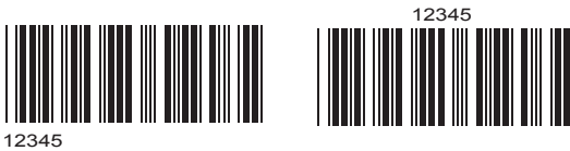
Left: Barcode with left-justified, bottom-positioned human-readable characters. Right: Barcode with center-justified, top-positioned human-readable characters.
