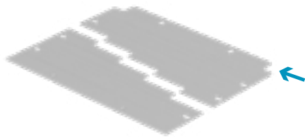
Integral Joint Strip Detail - Straight Ladder Covers for straight ladder have an integral joint strip on one end
