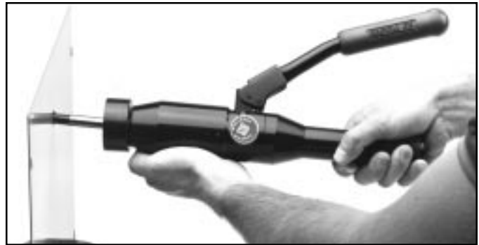
4. Turn release valve knob counterclockwise, to make sure the draw stud is fully extended. Insert stud through pilot hole.
