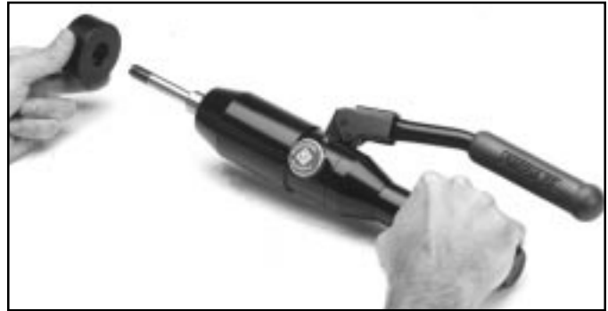
3. Thread 7/16" draw stud tightly into driver. Place die on draw stud.
