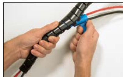
Simply slide the HAT applicator tool through the Helawrap cover.
