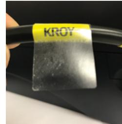
Step 3: Apply pressure to end of "tail" to ensure adhesive bond - **Job done!**
